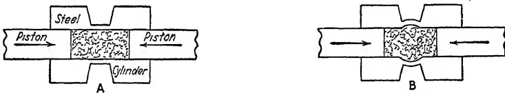
FIG. 428.—Diagrams illustrating the deformation of marble by great pressure. The left figure shows a section of a hollow cylinder in which a small cylinder of marble is fitted. The right figure shows the same after great pressure has been applied by movements of the pistons. The deformation took place slowly, resulting in shortening and bulging out of the marble cylinder. It is deformed but it is not crushed. (After Adams and Bancroft.)
